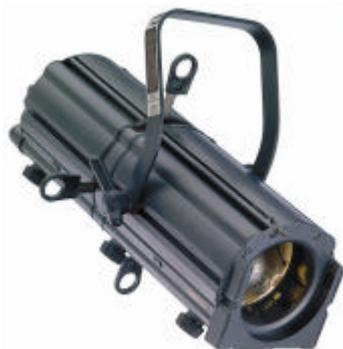
**A 500W / 650W variable beam profile providing precise beam control and pattern projection capability. The ellipsoidal optical system provides a high output beam with a centre peak. This can be made more even (2:1) by adjusting the position of the lamp in the reflector.**
